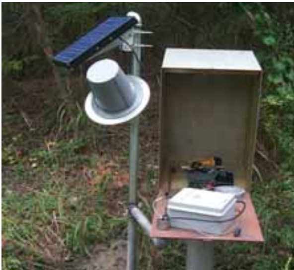
Figure 4.3 Monitoring well with satellite telemetry equipment.
